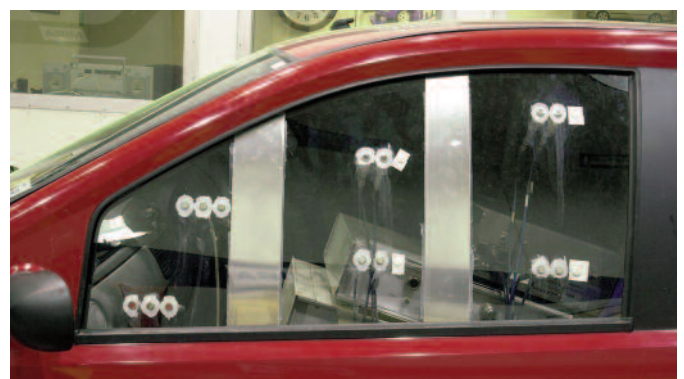
Experimental testing in MIRA's full-scale wind tunnel.
